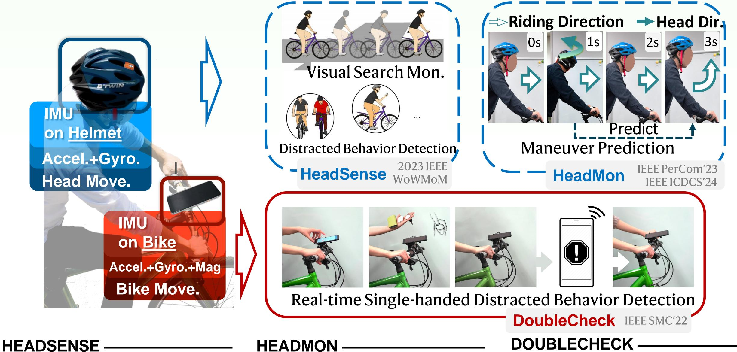
We present HeadSense, a helmet-based system that leverages the inertial motion unit (IMU) to recognize 4 distracted behaviors: checking handlebar-mounted devices, using smartphones, attracting to the roadside element, and abreast riding.
