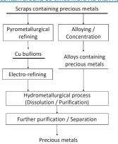
To dissolve precious metals into solution, the process
